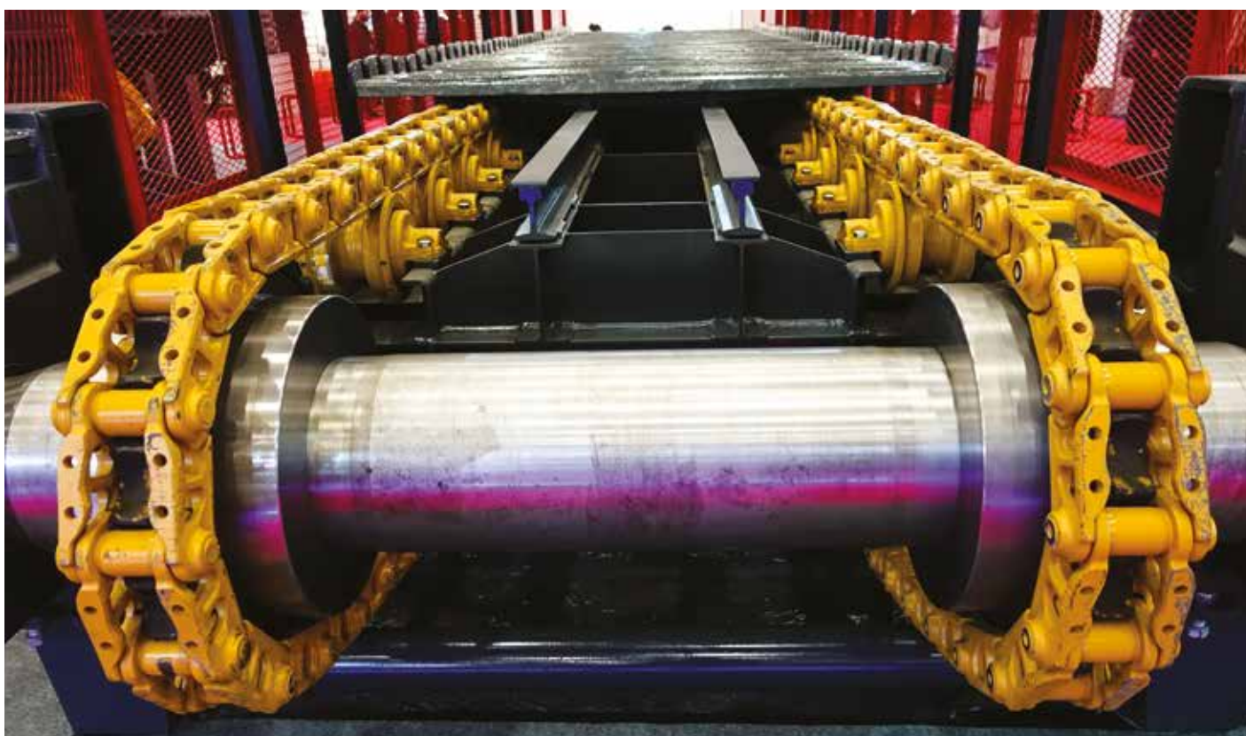
Locking conveyor chain wheels using SIT-LOCK® 4 COMPACT.
