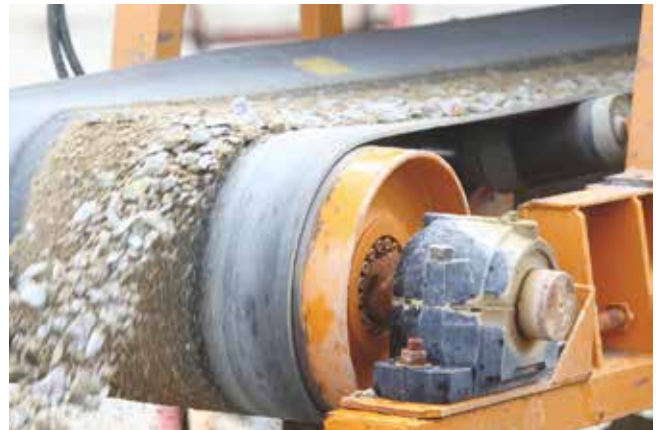
SIT-LOCK® 1 used for a conveyor belt pulley.
