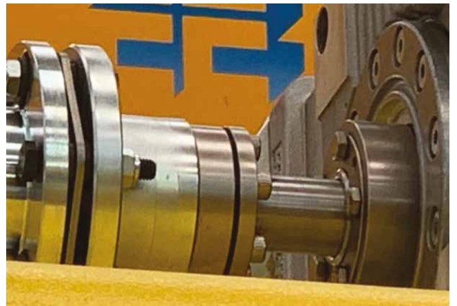
SIT-LOCK® 3 used for a disc coupling.
